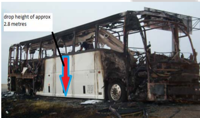
Figure 2.3: Height of Emergency Exit Windows
